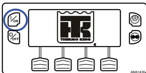
The startup screen (Figure 14, p. 39) appears while communications are established and the unit prepares for operation.
