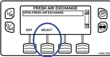
The Fresh Air Exchange door will open. To close the Fresh Air Exchange door press the SELECT Key again.
