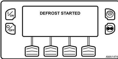
The display then shows the Defrost display. The bar indicator shows approximately how much time remains to complete the defrost cycle. The bar indicator shows that the defrost cycle is about 25% complete (Figure 55, p. 61).
