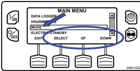
The first enabled Change Mode Menu selection will appear. To choose that function, press the SELECT Soft Key. To Scroll through the enabled features in the Change Mode Menu, press the UP and DOWN Soft Keys (Figure 120, p. 100).
