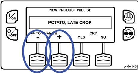
The YES and NO Keys confirm the product change (Figure 41, p. 53). When the desired product has been selected using the "+" and/or "-" Keys, press the YES Key to confirm and load the new product. If the product is changed using the "+" or "-" Keys, the change must be confirmed or rejected by pressing the YES or NO Key within 10 seconds of changing the product. A warning beep will sound for five seconds as a reminder.
