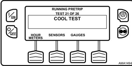
When all tests are complete, the results are reported as PASS, CHECK or FAIL (Figure 74, p. 74). If the results are CHECK or FAIL, the accompanying alarm codes will direct the technician to the cause of the problem.
