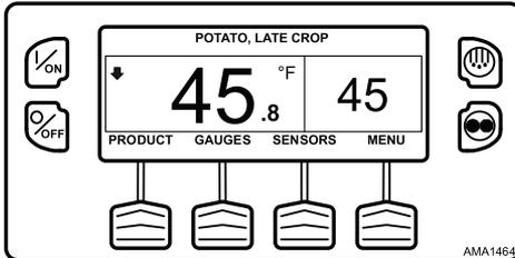
**Important:** If the named product is changed using the "+" or "-" Keys, the change must be confirmed or rejected by pressing the YES or NO Key within 10 seconds of changing the named product.
