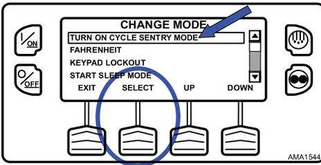
If the unit is running in Cycle Sentry Mode, press the SELECT Soft Key (Figure 122, p. 101) to turn off Cycle Sentry Mode as shown.
