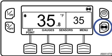
**Note:** Cycle Sentry Mode or Continuous Mode can also be selected using the Main Menu > Mode Submenu.
