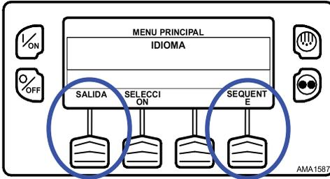
Repeat the process to select a different language. To select a different Main Menu item, press the NEXT (SIGUIENTE) Key. To return to the Standard Display, press the EXIT (SALIDA) Key.
