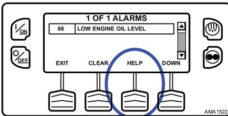
A help message will appear. Press the EXIT Key to return to the Alarms Menu (Figure 100, p. 89). Check the oil level and add oil as required, clear the alarm and restart the engine.
