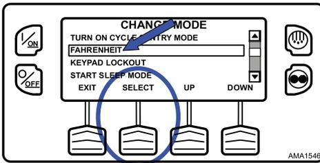
Choose the desired Temperature Units using the UP and DOWN Soft Keys and press the SELECT Soft Key to select the choice (Figure 124, p. 102).
