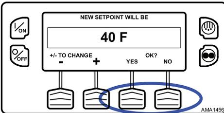
After the YES Key has been pressed, the display briefly shows PROGRAMMING NEW SETPOINT - PLEASE WAIT. The display then confirms the new setpoint for several seconds (Figure 36, p. 51).
