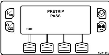
If the Pretrip Test results are CHECK or FAIL, the problem should be diagnosed and corrected by a Thermo King service technician before the unit is released for service.
