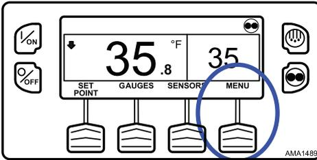
The Main Menu will appear. Press the UP or DOWN Key as required to choose the Gauges Menu. When the Gauges Menu is selected, press the SELECT Key to choose the Gauges Menu (Figure 102, p. 90).
