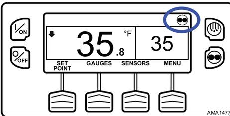
If allowed by OptiSet Plus, Cycle Sentry Mode or Continuous Mode is selected by pressing the Cycle Sentry/Continuous Key as shown (Figure 58, p. 63).
