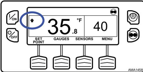
**Important:** If the setpoint is changed using the “+” or “-” Keys, the change must be confirmed or rejected by pressing the YES or NO Key within 10 seconds of changing the setpoint.
