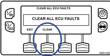
All ECU Faults and associated Thermo King Faults will be cleared.
