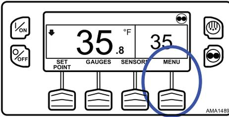
The Main Menu will appear. Press the UP or DOWN Key as required to choose the Adjust Brightness Menu. When the Adjust Brightness is selected, press the SELECT Key to choose the Adjust Brightness (Figure 136, p. 110).
