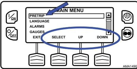
The display will briefly show PROGRAMMING PRETRIP MODE (Figure 70, p. 72). If the unit is not running, a Full Pretrip Test will be initiated. If the unit is running in either diesel or electric mode, a Running Pretrip Test will be performed.
