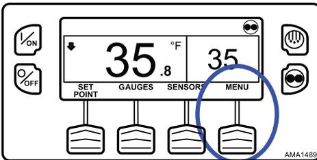
The Main Menu will appear. Press the UP or DOWN Key as required to choose the Clear All ECU Faults Menu. When the Clear All ECU Faults Menu is selected, press the SELECT Key to choose the Clear All ECU Faults Menu (Figure 142, p. 113).
