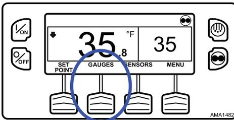
The first gauge display will appear. Press the NEXT and BACK Keys to scroll through the gauges. Pressing the LOCK Key will lock the current gauge on the display (Figure 63, p. 65).
