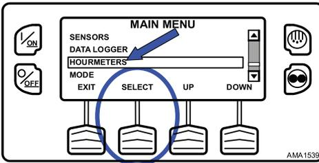
Press the NEXT or PREVIOUS Key to scroll through the hourmeters (Figure 117, p. 97).
