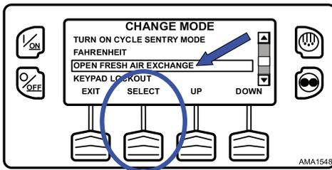
To open the Fresh Air Exchange door press the SELECT Key as shown below.
