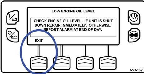
To return to the Main Menu press the EXIT Key. To return to the Standard display press the EXIT Key again.
