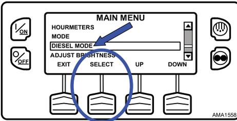
The new mode is confirmed for 10 seconds. The unit will start and run in Diesel Mode.
