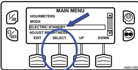
If the unit has standby power available and is turned on, the electric standby run screen will appear. The new mode is confirmed for 10 seconds. The unit will start and run in Electric Mode.
