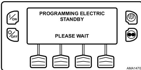
Electric Mode operation will briefly be confirmed. If unit operation is required the electric motor will start as shown previously under STARTING THE ELECTRIC MOTOR.
