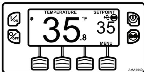
If an alarm condition (other than a Log Alarm) is present, the TemperatureWatch Display will not appear. If an alarm condition occurs while the TemperatureWatch Display is present, the display will return to the Standard Display.
