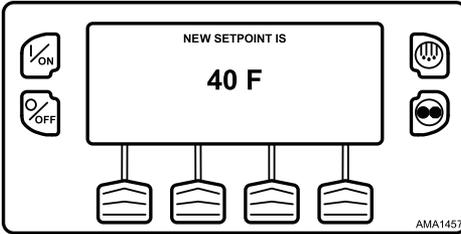
If the NO Key is pressed the display will briefly show SETPOINT NOT CHANGED and return to the Standard Display. The Standard Display will show the old setpoint.
