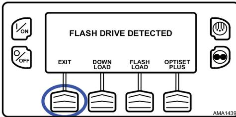
**Important:** *The engine start is not delayed by the Flash Drive Menu shown above. The engine start prompt will appear and the engine will start. After the engine is started the display will return to the Flash Drive Menu or the Standard Display.*
