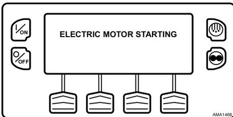
After the motor is started the display returns to the Standard Display of temperature and setpoint.
