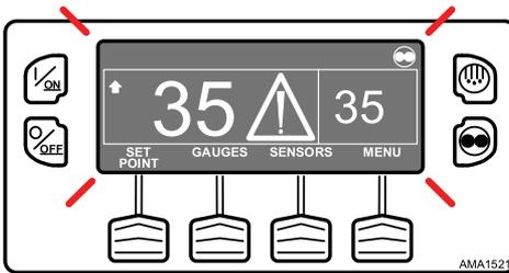
The Alarm Menu display will display the Shutdown Alarm Code. For additional information regarding the alarm shown on the display, press the HELP Key (Figure 99, p. 88).
