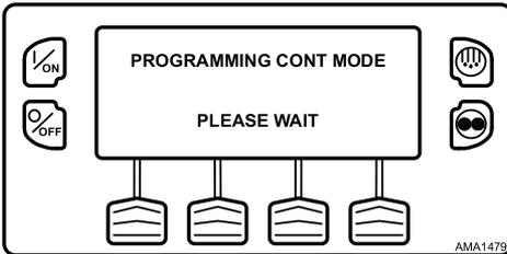
The new mode is confirmed for three seconds (Figure 60, p. 63).
