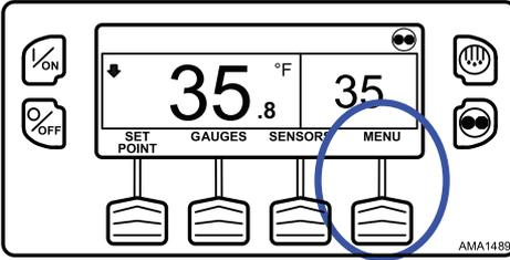
The Main Menu will appear. Press the UP or DOWN Key as required to choose the Mode Menu. When the Mode Menu is selected, press the SELECT Key to choose the Mode Menu (Figure 119, p. 100).
