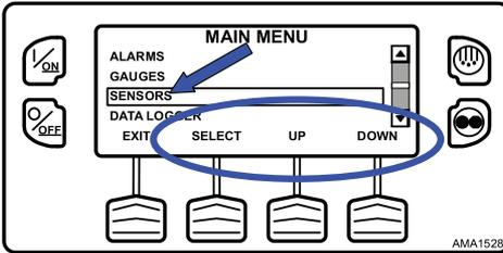
The first sensors display will appear. Press the NEXT and BACK Keys to scroll through the sensors and I/O conditions. Pressing the LOCK Key will lock the current sensor on the display (Figure 106, p. 92).
