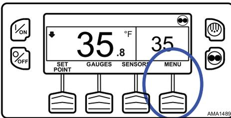
From the Main Menu choose Electric Standby and press the SELECT Soft Key (Figure 131, p. 107).
