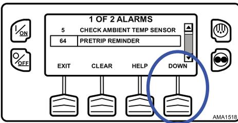
If the alarm situation has been resolved, press the CLEAR Key to clear the alarm (Figure 96, p. 87).
