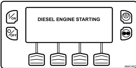
After the engine is started, the display returns to the Standard Display of temperature and setpoint.
