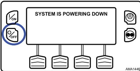
The display briefly shows OFF (Figure 26, p. 45) and then goes blank. To start the unit again, press the ON Key.
