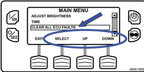
The Clear All ECU Faults Prompt will appear. To clear all ECU Faults and associated Thermo King Faults, press the CLEAR Soft Key (Figure 143, p. 113).
