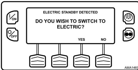
If NO is selected, the unit will continue to operate in Diesel Mode. If YES is selected, the display will briefly show the screen (Figure 50, p. 58).
