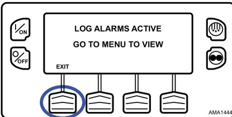
**Note:** The Alarm Icon does not appear on startup with log alarms present.
