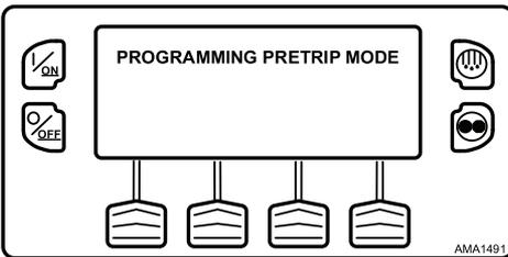
If all alarms were not cleared, a prompt appears (Figure 71, p. 73). Exit the Pretrip Test, clear all alarms, and repeat the Pretrip Test.
