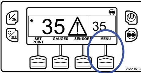
The Main Menu will appear. Press the UP or DOWN Key as required to choose the Alarms Menu (Figure 93, p. 86). When the Alarms Menu is shown, press the SELECT Key to select the Alarms Menu.
