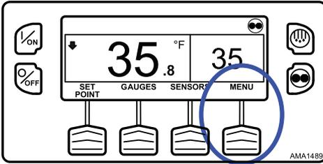
The Main Menu will appear. Press the UP or DOWN Key as required to choose the Time Menu. When the Time Menu is selected, press the SELECT Key to choose the Time Menu (Figure 139, p. 111).
