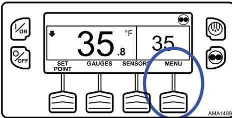
The Main Menu will appear. Press the UP or DOWN Key as required to choose the Data Logger Menu. When the Data Logger Menu is selected, press the SELECT Key to choose the Data Logger Menu (Figure 108, p. 93).
