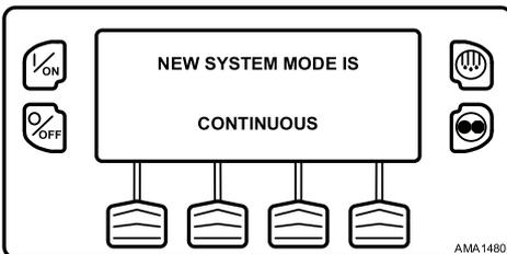
The display then returns to the Standard Display. In the example shown (Figure 61, p. 64), the absence of the Cycle Sentry Icon indicates that the unit is running in Continuous Mode.
