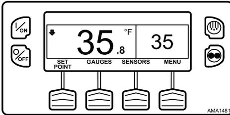
Pressing the Cycle Sentry/Continuous Key again allows the operator to change back to Cycle Sentry Mode operation.
