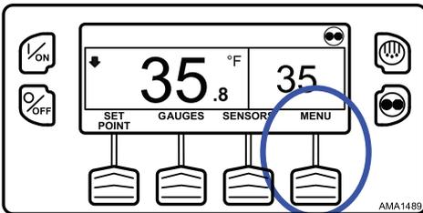
The Main Menu will appear. Press the UP or DOWN Key as required to choose the Sensors Menu. When the Sensors Menu is selected, press the SELECT Key to choose the Sensors Menu (Figure 105, p. 92).
