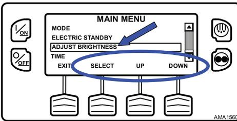
The Display Brightness menu will appear as shown. Press the UP or DOWN Soft Keys to select the desired display brightness. When the desired brightness is shown, press the SELECT Soft Key to confirm the choice (Figure 137, p. 110).
