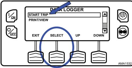
**Note:** The start of trip marker is sent to both the CargoWatch and ServiceWatch data loggers.
