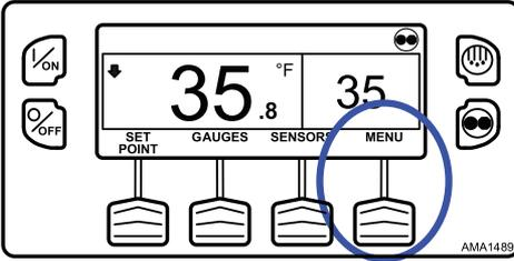
The Main Menu will appear. Press the UP or DOWN Key as required to choose the Pretrip Menu. When the Pretrip Menu is shown, press the SELECT Key to start a Pretrip Test (Figure 69, p. 72).
