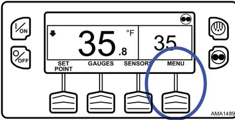
The Main Menu will appear. Press the UP or DOWN Key as required to choose the Hourmeter Menu. When the Hourmeter Menu is selected, press the SELECT Key to choose the Hourmeter Menu (Figure 116, p. 97).
