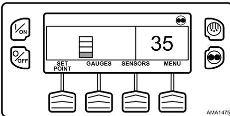
If conditions do not allow a defrost cycle, the display shown (Figure 56, p. 61) will briefly appear. The display will then return to the Standard Display.
