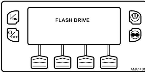
The FLASH DRIVE DETECTED and the Flash Drive Menu will appear on the display (Figure 16, p. 40). The display will be shown for about 30 seconds and then the Standard Display will appear. To go to the Standard Display, immediately press the EXIT Soft Key.
