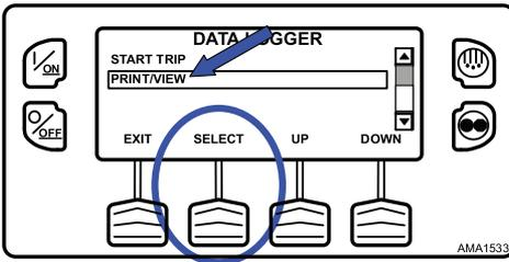
The Print Data Menu will appear. The first Print Data Menu allows the operator to print a Delivery Ticket using a hand held printer. Pressing the SELECT Key will print the ticket (Figure 111, p. 95). The Delivery Ticket is a short ticket that shows delivery specific details including the current temperature. A Sample Delivery Ticket is shown (Figure 112, p. 95).
