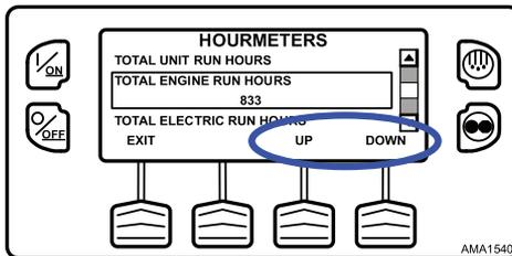
Hourmeter names and definitions are shown below in the order they appear. Only hourmeters enabled in the Guarded Access Menu will be shown. To return to the Standard Display, press the EXIT Key.
