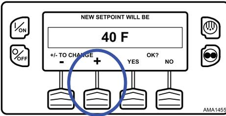
The YES and NO Keys (Figure 35, p. 50) confirm the setpoint change. When the desired setpoint has been selected using the “+” and/or “-” Keys, press the YES Key to confirm and load the new setpoint. If the setpoint is changed using the “+” or “-” Keys, the change must be confirmed or rejected by pressing the YES or NO Key within 10 seconds of changing the setpoint. A warning beep will sound for five seconds as a reminder.
