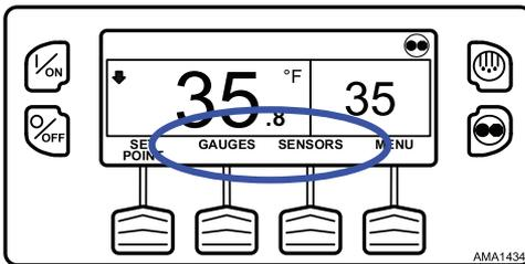
The functions of these two keys can be changed as required for customer convenience. The functions of these two soft keys on the Standard Display can be re-assigned to any of the following functions using the Guarded Access > Main Menu Configuration menu:
