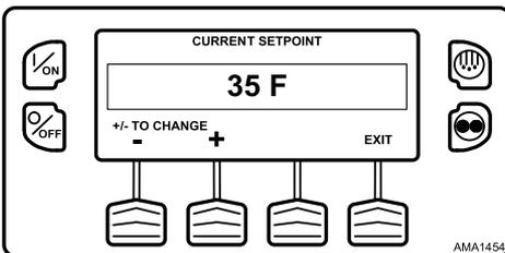
The “-” and “+” Keys are used to increase or decrease the setpoint until the desired setpoint is shown. The setpoint has been changed to 40 F using the “+” Key (Figure 34, p. 50).
