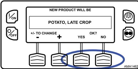
After the YES Key has been pressed, the display briefly shows PROGRAMMING NAMED PRODUCT - PLEASE WAIT. The display then confirms the new setpoint for several seconds (Figure 42, p. 54).
