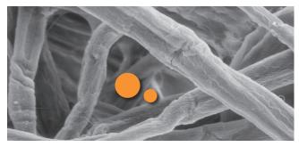
Cellulose fibers are larger and have larger spaces between the fibers, causing contaminant to load in the depth of the media and plug the airflow path; resulting in higher restriction and less capacity.
