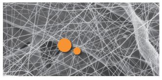
The fibers in the Thermo King filter media have submicron diameter and small interfiber spaces, which result in more contaminant being captured on the surface of the media and lower restriction.
