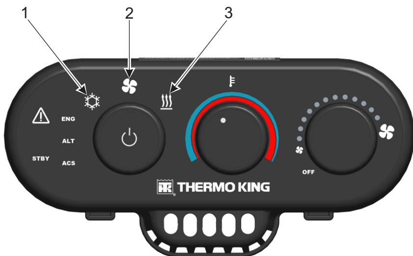
Figure 12. Rotate Mode Selector Knob to Desired Operating Mode
