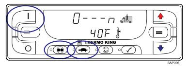
When Keypad Lockout is turned on, only the ON and OFF Keys are functional. All other keys are locked out. Pressing any key other than the ON Key and OFF Key will cause the box temperature to display [0 - - - n]. When the key is released, the display will return to the Standard Display of box temperature and setpoint.
