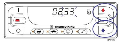
Press the Enter Key to load the Date and Time. The time shown is 8:33 AM and date is January 27th.
