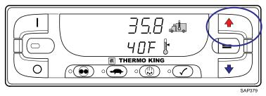
When the desired setpoint has been selected using the UP ARROW Key or DOWN ARROW Key, the ENTER Key must be pressed to confirm and load the new setpoint.
