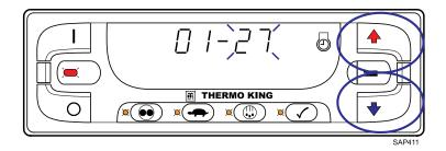
Press the Enter key to display the Time. The Hour setting will flash indicating it can be changed. The hours shown in 24 Hour clock format are "14", which is the same as 2 PM.
