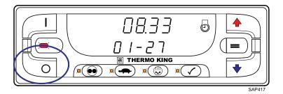
Verify the Date and Time is correct displaying the current date and time as shown under Displaying Date and Time. Date and time can also be checked using WinTrac 5.3 or later.
