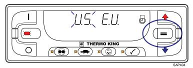
Using the Up Arrow Key and/or Down Arrow Key, select the flashing display to either "US" or "EU" as desired.
