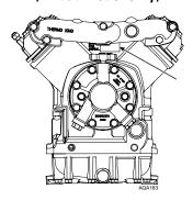
Figure 44. Unit Serial Number Plate Located on Frame
