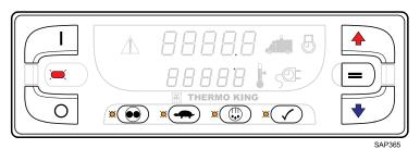
There are amber LED indicators located next to each of the four function keys below the display. The LED will glow amber when that function is active. A red LED indicator is located between the ON Key and OFF Key at the left side of the display. This indicator will glow if Alarm Code 91 Check Electric Ready Input occurs. It will also illuminate if a 15 pin Thermo King Data Cable is connected to the serial port on the back of the Base Controller.
