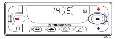
Using the Up Arrow Key and/or Down Arrow Key, select the desired Minutes. The minutes shown are now 33 minutes past the hour.
