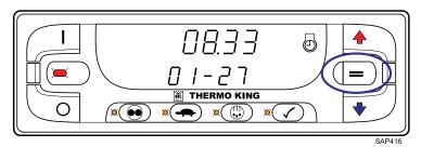
To leave the Date and Time Display press the Off Key. The displays will also time out after one minute.
