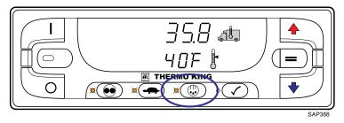
Important: During the defrost cycle, the box temperature will rise toward 50° F (10°C). This is normal and is caused by the defrost cycle warming the evaporator coil. Since the damper door is closed during the defrost cycle, this warm air is not allowed to pass into the truck box.
