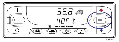
The new setpoint of 40°F (4.4°C) will remain on the display after the ENTER Key has been pressed.
