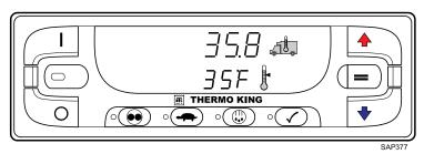
Pressing the OFF Key stops unit operation. The unit shuts down immediately and the display goes blank. To start the unit again, press the ON Key (Figure 15, p. 33).
