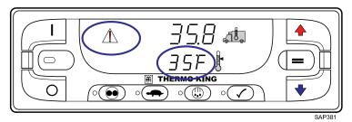
Notice that the setpoint has returned to the old setpoint of 35°F (1.6°C) and the Alarm Icon has lighted indicating that Alarm Code 127 Setpoint Not Entered is set.
