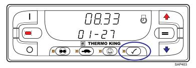
When the current Date and Time is shown on the display, press and hold the Enter key to display US - EU.
