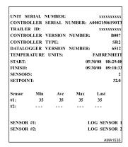
Pressing the DOWN Key allows the operator to print a Trip Ticket using a hand held printer. Press the SELECT Key to print the ticket (Figure 113, p. 95). The Trip Ticket is a long ticket that shows details for the current trip including a temperature history. The Trip Ticket is also called a Journey Ticket. A sample Trip Ticket is shown (Figure 114, p. 96).
