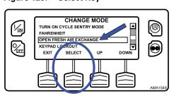
To open the Fresh Air Exchange door press the SELECT Key as shown below.
