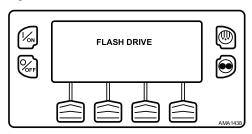
The FLASH DRIVE DETECTED and the Flash Drive Menu will appear on the display (Figure 16, p. 40). The display will be shown for about 30 seconds and then the Standard Display will appear. To go to the Standard Display, immediately press the EXIT Soft Key.
