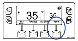
The Main Menu will appear. Press the UP or DOWN Key as required to choose the Data Logger Menu. When the Data Logger Menu is selected, press the SELECT Key to choose the Data Logger Menu (Figure 108, p. 93).
