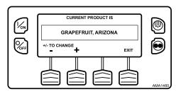
The "-" and "+" Keys are used to change the Named Product until the desired product is shown. The product has been changed to Potato, Late Crop (Figure 40, p. 53).
