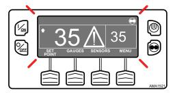
The Alarm Menu display will display the Shutdown Alarm Code. For additional information regarding the alarm shown on the display, press the HELP Key (Figure 99, p. 88).
