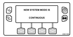
The display then returns to the Standard Display. In the example shown (Figure 61, p. 64), the absence of the Cycle Sentry Icon indicates that the unit is running in Continuous Mode.
