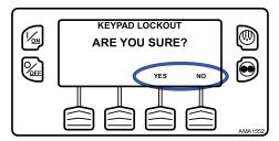
If the YES Soft Key was pressed, Keypad Lockout is active. Repeat the process to turn the Keypad Lockout feature off.
