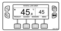
Important: If the named product is changed using the "+" or "-" Keys, the change must be confirmed or rejected by pressing the YES or NO Key within 10 seconds of changing the named product.
