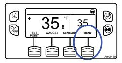
From the Main Menu choose Diesel Mode and press the SELECT Soft Key (Figure 134, p. 109).
