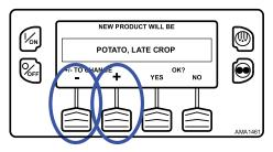
The YES and NO Keys confirm the product change (Figure 41, p. 53). When the desired product has been selected using the "+" and/or "-" Keys, press the YES Key to confirm and load the new product. If the product is changed using the "+" or "-" Keys, the change must be confirmed or rejected by pressing the YES or NO Key within 10 seconds of changing the product. A warning beep will sound for five seconds as a reminder.
