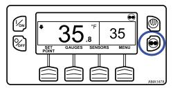
**Note:** Cycle Sentry Mode or Continuous Mode can also be selected using the Main Menu > Mode Submenu.
