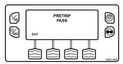
If the Pretrip Test results are CHECK or FAIL, the problem should be diagnosed and corrected by a Thermo King service technician before the unit is released for service.
