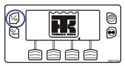
The startup screen (Figure 14, p. 39) appears while communications are established and the unit prepares for operation.
