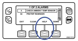
If necessary to view all alarms, scroll down using the DOWN Key (Figure 95, p. 87).
