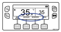
The functions of these two keys can be changed as required for customer convenience. The functions of these two soft keys on the Standard Display can be re-assigned to any of the following functions using the Guarded Access > Main Menu Configuration menu:
