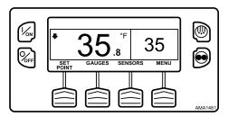
Pressing the Cycle Sentry/Continuous Key again allows the operator to change back to Cycle Sentry Mode operation.
