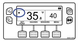
Important: If the setpoint is changed using the "+" or "-" Keys, the change must be confirmed or rejected by pressing the YES or NO Key within 10 seconds of changing the setpoint.
