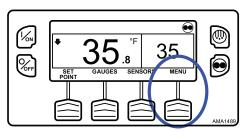
If a properly configured USB Flash Drive is connected to the Flash Drive Only USB Port on the Control Panel, the Flash Drive Menu will appear as a Main Menu selection. Press the UP or DOWN Key as required to choose the Flash Drive Menu. When the Flash Drive Menu is shown, press the SELECT Key to select the Flash Drive Menu (Figure 77, p. 76).
