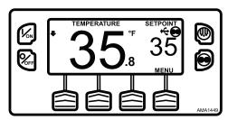
If an alarm condition (other than a Log Alarm) is present, the TemperatureWatch Display will not appear. If an alarm condition occurs while the TemperatureWatch Display is present, the display will return to the Standard Display.
