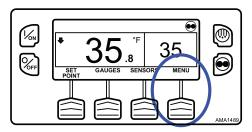
The Main Menu will appear. Press the UP or DOWN Key as required to choose the Gauges Menu. When the Gauges Menu is selected, press the SELECT Key to choose the Gauges Menu (Figure 102, p. 90).
