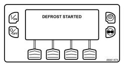
The display then shows the Defrost display. The bar indicator shows approximately how much time remains to complete the defrost cycle. The bar indicator shows that the defrost cycle is about 25% complete (Figure 55, p. 61).
