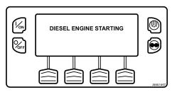
After the engine is started, the display returns to the Standard Display of temperature and setpoint.
