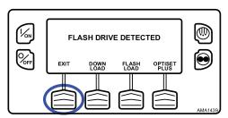
Important: The engine start is not delayed by the Flash Drive Menu shown above. The engine start prompt will appear and the engine will start. After the engine is started the display will return to the Flash Drive Menu or the Standard Display.
