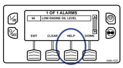
A help message will appear. Press the EXIT Key to return to the Alarms Menu (Figure 100, p. 89). Check the oil level and add oil as required, clear the alarm and restart the engine.
