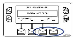
After the YES Key has been pressed, the display briefly shows PROGRAMMING NAMED PRODUCT - PLEASE WAIT. The display then confirms the new setpoint for several seconds (Figure 42, p. 54).
