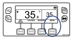
The Main Menu will appear. Press the UP or DOWN Key as required to choose the Clear All ECU Faults Menu. When the Clear All ECU Faults Menu is selected, press the SELECT Key to choose the Clear All ECU Faults Menu (Figure 142, p. 113).
