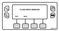
If the HELP Soft Key is pressed, the display shown (Figure 80, p. 78) will appear.
