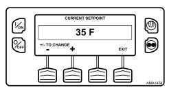
The "-" and "+" Keys are used to increase or decrease the setpoint until the desired setpoint is shown. The setpoint has been changed to 40 F using the "+" Key (Figure 34, p. 50).
