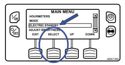
If the unit has standby power available and is turned on, the electric standby run screen will appear. The new mode is confirmed for 10 seconds. The unit will start and run in Electric Mode.
