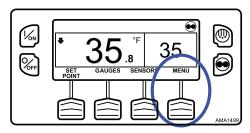
The Main Menu will appear. Press the UP or DOWN Key as required to choose the Sensors Menu. When the Sensors Menu is selected, press the SELECT Key to choose the Sensors Menu (Figure 105, p. 92).
