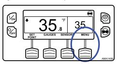
The Main Menu will appear. Press the UP or DOWN Key as required to choose the Time Menu. When the Time Menu is selected, press the SELECT Key to choose the Time Menu (Figure 139, p. 111).
