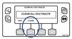
All ECU Faults and associated Thermo King Faults will be cleared.
