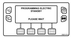
Electric Mode operation will briefly be confirmed. If unit operation is required the electric motor will start as shown previously under STARTING THE ELECTRIC MOTOR.
