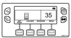
If conditions do not allow a defrost cycle, the display shown (Figure 56, p. 61) will briefly appear. The display will then return to the Standard Display.
