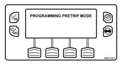
If all alarms were not cleared, a prompt appears (Figure 71, p. 73). Exit the Pretrip Test, clear all alarms, and repeat the Pretrip Test.
