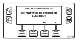
If NO is selected, the unit will continue to operate in Diesel Mode. If YES is selected, the display will briefly show the screen (Figure 50, p. 58).
