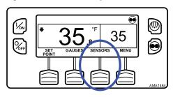
The first sensor display will appear. Press the NEXT and BACK Keys to scroll through the sensors. Pressing the LOCK Key will lock the current sensor on the display (Figure 65, p. 67).
