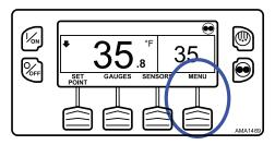
The Main Menu will appear. Press the UP or DOWN Key as required to choose the Pretrip Menu. When the Pretrip Menu is shown, press the SELECT Key to start a Pretrip Test (Figure 69, p. 72).
