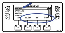
The display will briefly show PROGRAMMING PRETRIP MODE (Figure 70, p. 72). If the unit is not running, a Full Pretrip Test will be initiated. If the unit is running in either diesel or electric mode, a Running Pretrip Test will be performed.
