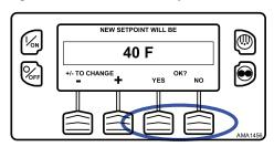
After the YES Key has been pressed, the display briefly shows PROGRAMMING NEW SETPOINT - PLEASE WAIT. The display then confirms the new setpoint for several seconds (Figure 36, p. 51).
