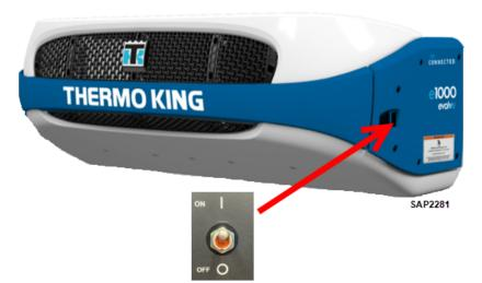
Figure 9. Unit Service Switch location shown
