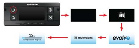
To turn the HMI Controller Off, press and hold the Power button for five seconds from any screen. Shutdown and HMI Off will be displayed briefly and Switching Off HMI will appear prior to the HMI turning off and the unit shutting down.
