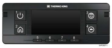
On/Off: Used to turn the unit on/off. A short press will turn the unit on. A long press of five seconds will switch off the HMI and shut down the unit. Refer to "Start/ Shutdown Sequence," p. 26.
