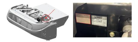
**Vehicle**: A second unit nameplate is typically located on the inside driver's door jamb. This nameplate also lists the unit serial number, model number, and bill of material number.
