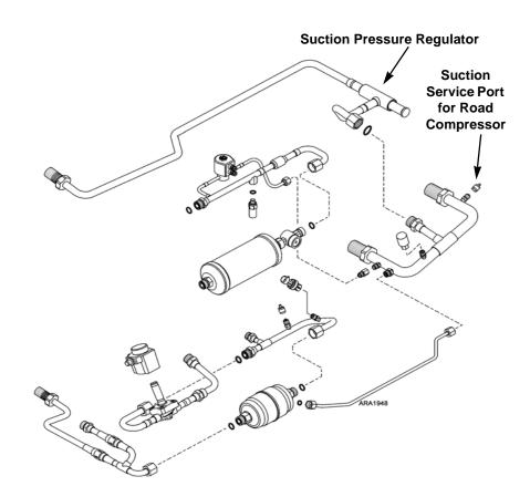
Typical V-520 RT Refrigeration Module Components
