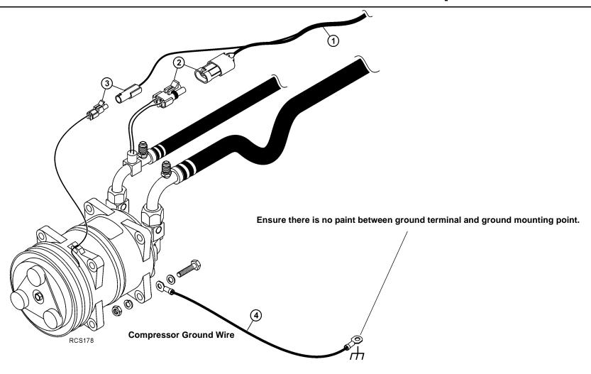
IMPORTANT: Failure to install the compressor ground wire to the chassis may result in intermittent clutch operation and premature clutch failure!
