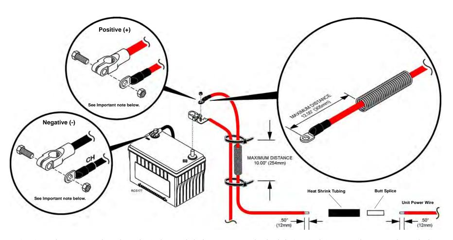
IMPORTANT: The ring terminals used must be sized to match the battery power stud or lug bolt. Oversized ring terminals can contribute to high resistance resulting in the fuse overheating and failure.
