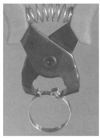
Nose of the pliers should be firmly seated under the assembly bump and lock latch.
