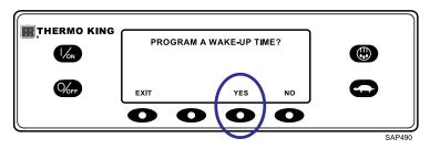
The display will prompt the operator for the DAY the unit is to restart in normal operation. In the example shown (Figure 102, p. 79), Monday has been chosen. Press the YES key to confirm the DAY.
