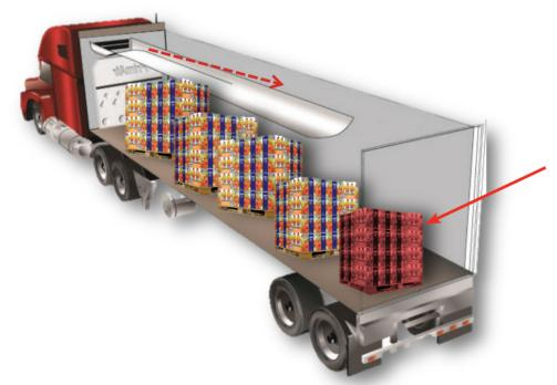
Precedent's high airflow can make a difference, reaching pallets in the back of the trailer.
