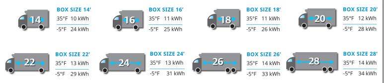
Assuming 3" of insulation for 35°F, and 4" for -5°F at an 80°F ambient; ten door openings for ten minutes each per day on a ten hour route with box pre-cooled to setpoint; box dimensions of 96'W and 96''H on trucks 10' and over in length.
