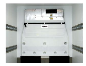
Reduce short-cycling and maintain uniform product temperatures with this easy-to-use bulkhead. It takes less than one minute to remove the bulkhead to access the refrigeration unit. Replace pallet stops as needed without replacing entire bulkhead. No tools needed.
