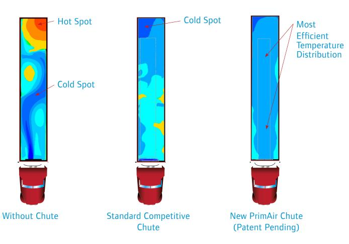
Results based on Thermo King CFD analysis on loaded trailer.
