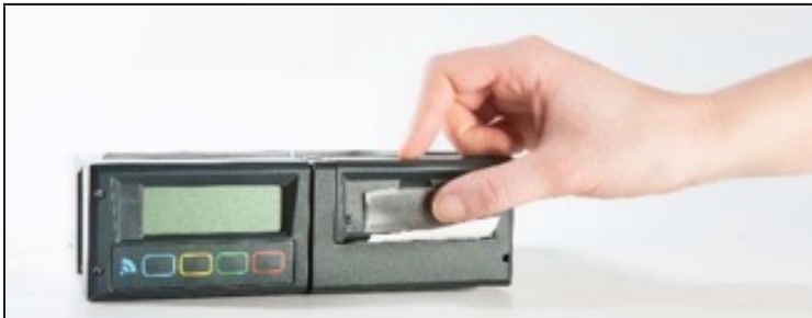
5.) Close the flap only after the printer is fully inserted.
