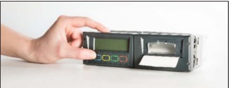
6.) Test if the paper roll is properly replaced by printing any ticket.
