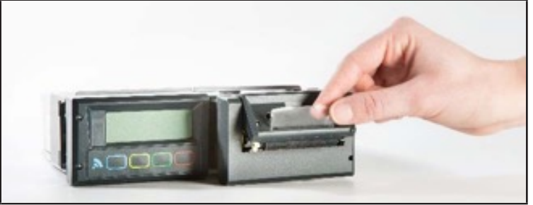
2.) Printer slides forward and can be pulled out. Now you can remove the empty roll
