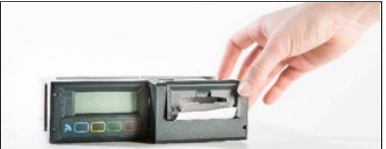
4.) After changing the paper please install the printer with the flap open.
