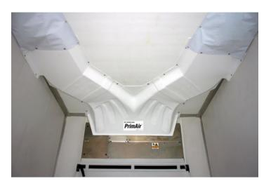
The PrimAir Split Air Chute System is designed to provide uniform temperature throughout the entire trailer. The unique diverter evenly distributes air to each side chute, which then guides the air to the rear of the trailer.
