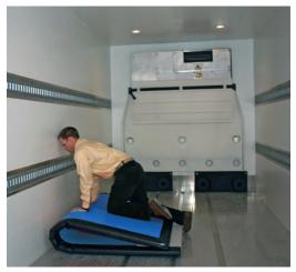
The PrimAir Insulated Bulkhead is designed and constructed for exceptional durability at an extremely light weight. Easy on loaders and easy on drivers.
