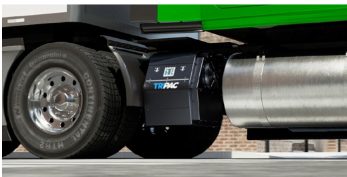
Figure 1: APUs provide energy for essential truck functions while stationary—such as HVAC, lighting, appliances, and other driver comforts—to prevent the need for inefficient engine idling.
