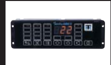
Microprocessor Controller/ CAN Bus Communications
