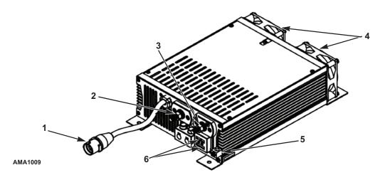
Figure 1: Converter/Charger Components
