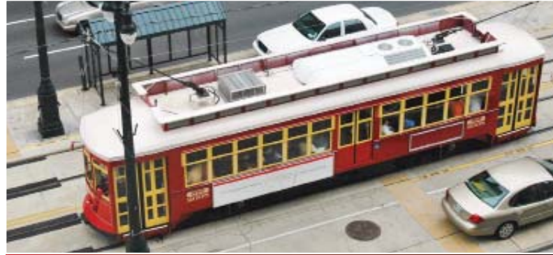
Streetcar 2008 on a test run on Canal Street. The Thermo King air conditioning unit is visible on the roof.
