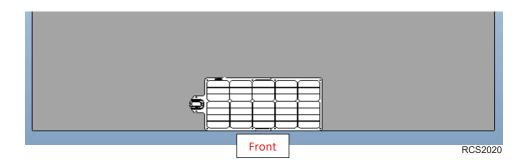
Thermo King does not recommend more than one 40W panel (unless there are specific space restrictions) as going to a single 110W solar panel is a better solution.
