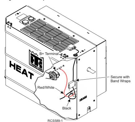
Figure 10. Solar panel electrical connections shown
