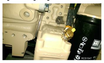
11. Coil up the extra harness length in front of the starter and secure with band wraps.
