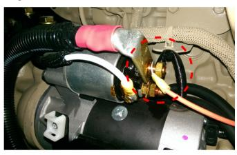
10. Attach the black wire to the engine block ground stud behind the oil filter.
