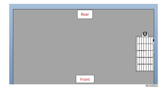
Thermo King does not recommend more than one 40W panel (unless there are specific space restrictions) as going to a single 110W solar panel is a better solution.
