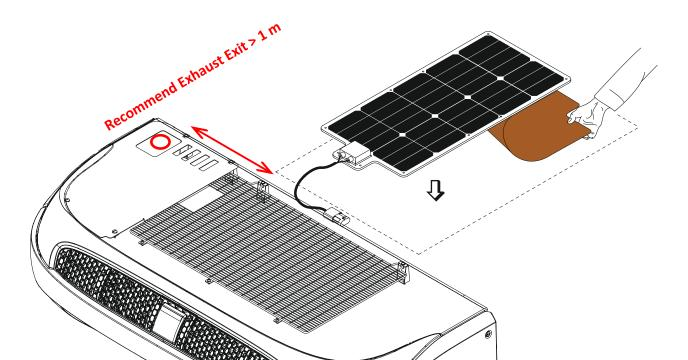
Figure 20. Typical installation on roof of cargo box shown
