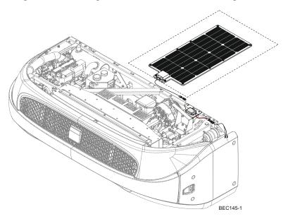
6. Safely route, secure, and connect the red wire (B+) to alternator B+ terminal.
