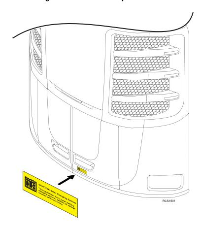
Figure 19. Install nameplate on unit
