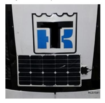
Figure 11. Correct panel location shown
