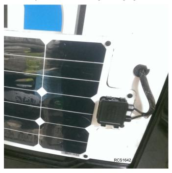
7. Connect the extension harness (401293) and route the harness near the top of the roadside door hinge. Secure using band wraps and ensure the door does not bind when closing.
