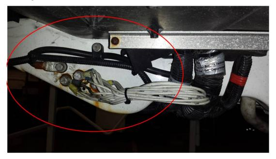
8. Clean surface and attach supplied nameplate on the battery box unit near the solar panel terminal connection. The label must be visible to servicing technicians to warn of additional charging sources.
