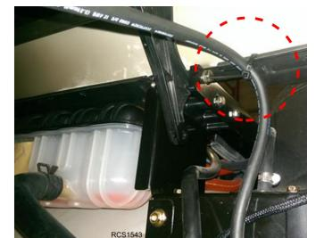
Figure 13. Proper harness routing shown
